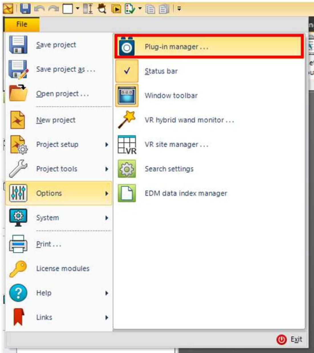
In the Plug-in Manager, click “Install plugin-in...”. Navigate to the location of the provided \*.pip file and click “Open”.
